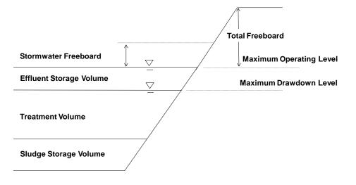
Figure 1. Parts of a Treatment Lagoon (from F-1738, Lagoons for Livestock Waste Treatment. Oklahoma Cooperative Extension Service).
