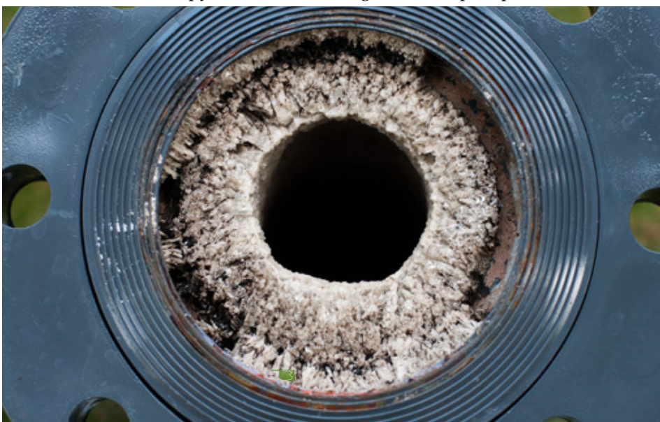
A struvite clogged sewer line (from UBC civil engineering news)
