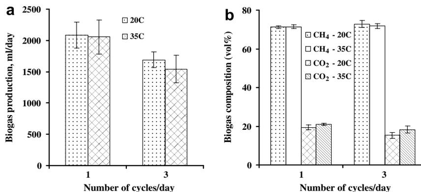
Fig. 3. Effect of cycle-frequency and temperature on the biogas production and quality.
